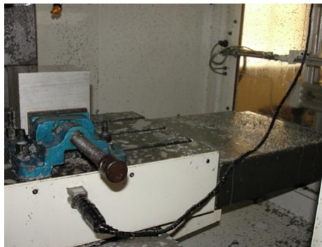
Figure 4.1 the vibration accelerometer placed on work table.
